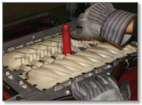
Matchplate with FDM insert in molding machine
