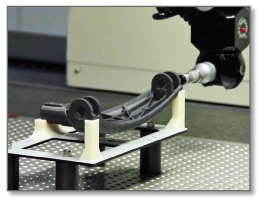
Oreck uses an FDM surrogate first article on an FDM fixture to conduct CMM programming.
