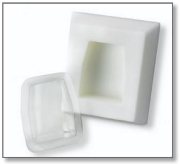
Thermoformed packaging cover and FDM mold
