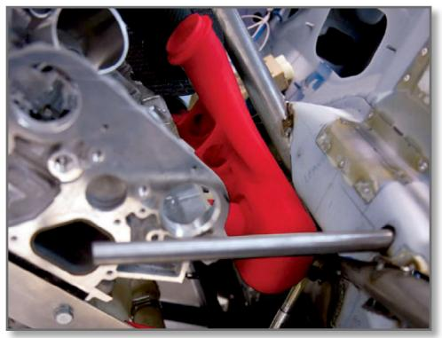
Red FDM material in assembly mockup quickly identifies surrogate part
