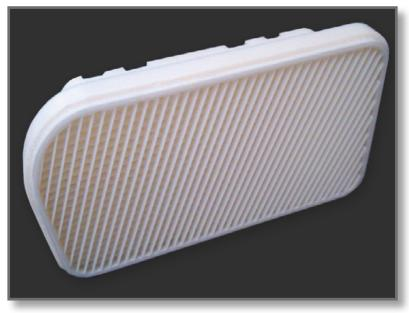
FDM paper pulp tool with sparse fill to enable vacuum forming
